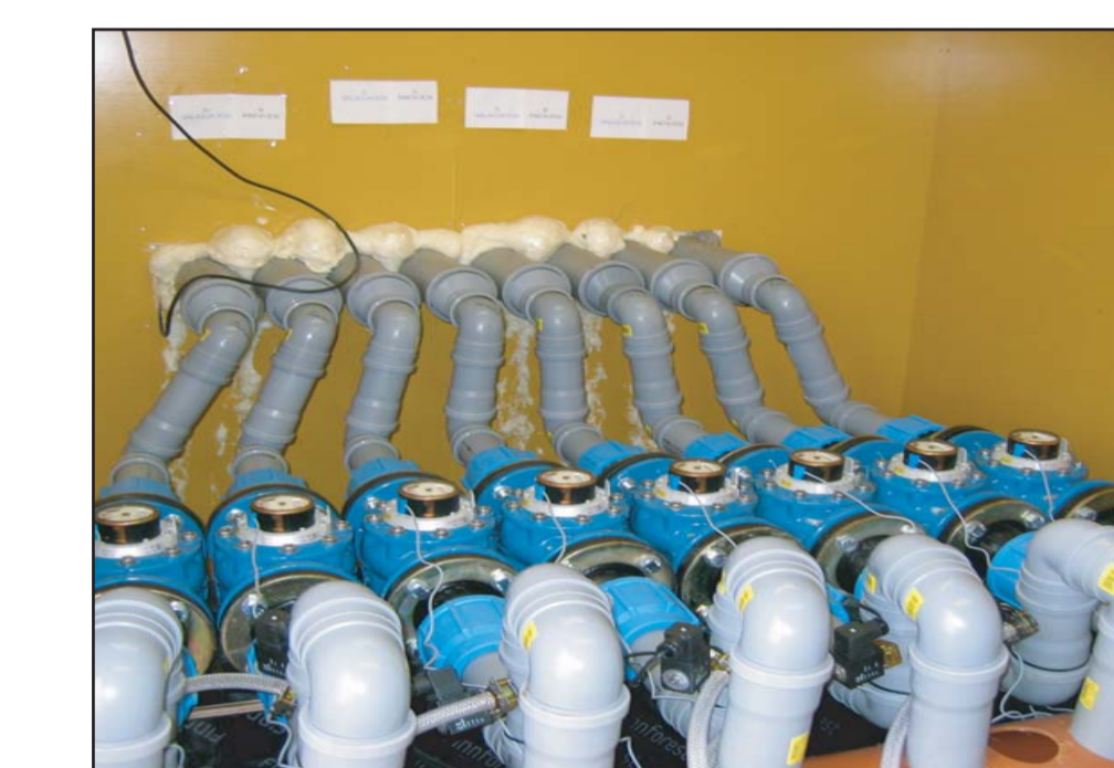
The subsurface and surface runoff waters from each plot are measured. The flow-weighted water samples are collected through an electromagnet valve to plastic containers for further sampling and chemical analyses.
