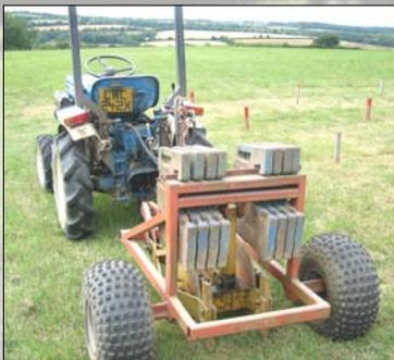
Fig. 3. Disc cutter used to make shallow injection slots
