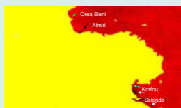
Fig. 3 Colour composite 4,2,1 (R,G,B) of the Landsat 7 ETM+ image with bands to actual and histogram logarithmic transform. The dry land has been masked out. Springs Orea Eleni, Almiri, Korfou, Selonda and two possible unidentified (so far) ground water discharges are being displayed.
