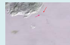
Fig. 7 False colour composite (13,10,14) R,G,B of thermal bands that display the submarine spring near Agia Irini (darker grey areas indicate lower temperature ground water discharge into the higher temperature sea water).
