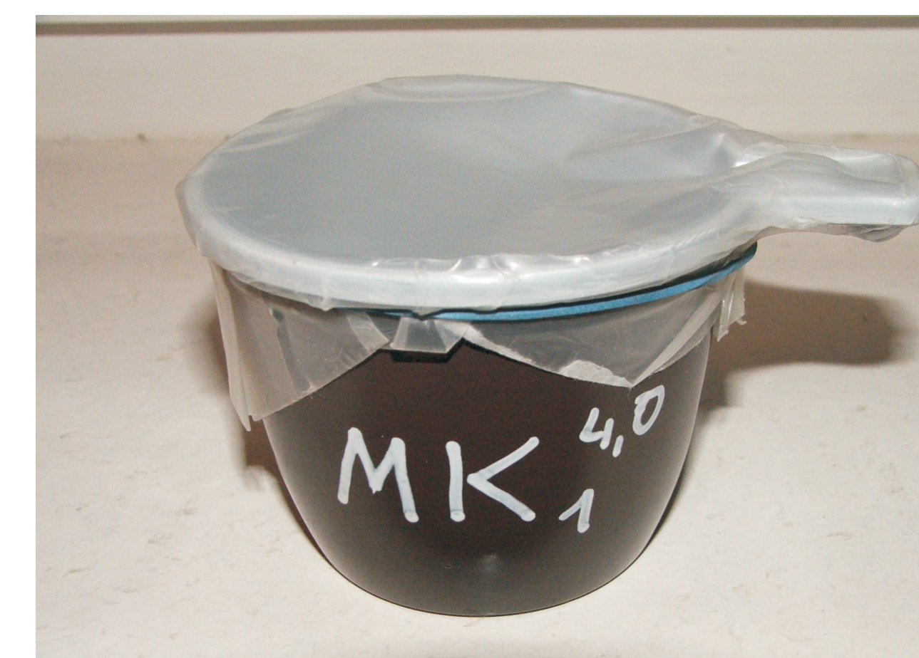
Pic. 2. The plastic cup with soil sample closed by PARAFILM M in the laboratory experiment (2001).
